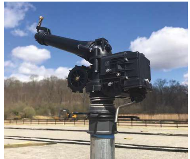
Turbina ST-1200-BR Instalada
